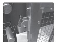
3.3 Pull the locks back on either side and lower the guard all the way down.
