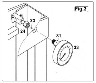
3.1.4. Assemble the gauge fitting (31) the nylon ring (32), (which fits between the gauge and the gauge fitting see fig.4), and the gauge (33). Twist the gauge as tight as possible to prevent it from leaking. Then the gauge and gauge fitting are fitted to the manifold (24).
