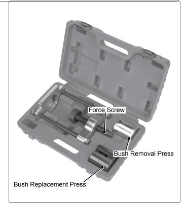
Force screw maximum load 150Nm. Exceeding this load will shorten the life of the force screw. The force screw is considered to be a consumable item and is NOT covered under warranty.
