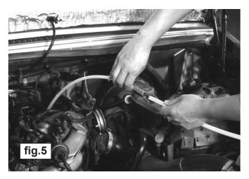
4.3 Insert the appropriate extracting probe into the dipstick tube making sure it reaches the bottom of the sump. Connect the extracting probe to the extension tube using the black or red soft plastic adaptor. The tubes are a push fit into the adaptor.
