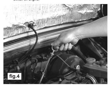
**4.2** Remove the oil dipstick from the engine.
