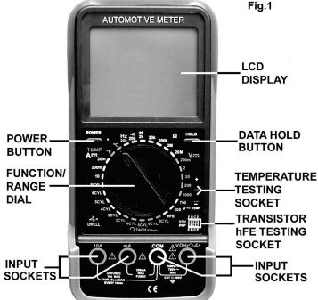
Maximum Display: 1999 counts - (3 1/2 digits) LCD display with automatic polarity indication.
