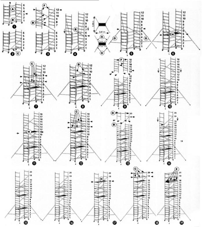
diagonal on the same frame on the second rung on the other side. The last diagonal is to be placed on the top rung of the second end frame (WARNING: Make sure that everything is the right way round as per the sketch!)
