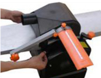
4.2.7 Remove chute from underneath table and place on top over blade
