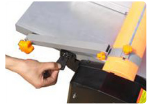
4.1.6 Insert the keys into the cut-outs, locking the chute into place.
