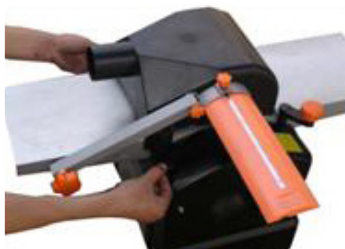
4.2.8 Locate the two keys on the chute and align with the cut-outs on the table and insert the keys.
