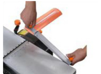
4.2.6 Set the safety guard at its uppermost position and fasten the set screw.
