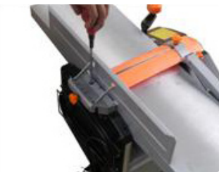
4.2.1 Remove the set bolt on the fence seat.
