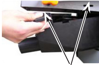
4.1.5 The chute should be positioned to allow both the keys to align with the cut-outs on the table
