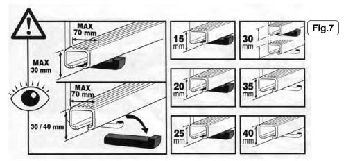
3.7. Check the dimensions of the roof bars fitted to your car in fig.7. Measure the section of your roof bars to see if the plastic hook bolt covers need to be fitted
