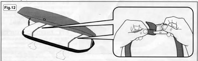
**3.13.** Use the two straps provided, threaded through the body of the fixing system (refer to 3.11.), to secure the load within the roofbox.
