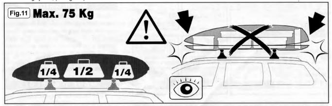
3.12. Distribute the load evenly in the roofbox. **DO NOT** place tall objects in the roofbox which will prevent it from closing correctly (see fig.11).
