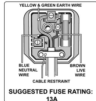
Double insulated products, which are always marked with this symbol
