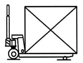
Lowering the truck. ( See fig.2 - L ) Before inserting the truck into the pallet ensure that the truck forks are in their lowest position by pulling the operating lever into the upper position and holding it there until the truck has settled down to the lowest level
