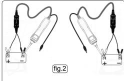
While the PP7 is in "Power While the PP7 is in "Power Mode", contact the probe tip to a NEGATIVE circuit. The green negative sign (-) The red positive sign (+) LED will light. If the audio feature is turned on, a low pitched tone will sound.
