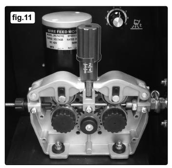
6.1 The wire feed mechanism has two separate grooved drive rollers and two separate pressure rollers. The pressure rollers are in separate housings which are held in place and acted upon by a single, central pressure adjustment knob as shown in fig.11 above. To access the drive mechanism pull the pressure adjustment knob forwards and allow it to hinge downwards. As you do so the pressure roller housings will spring upwards as shown in fig.12 below.
