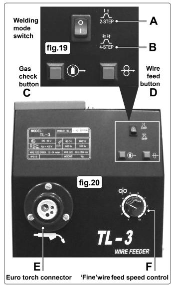
8.1.5 **Euro Torch Connector** (fig.20E) The torch should already be connected as described in Section 5.4. Ensure that the locking nut/ring is fully tightened and the wire has been fed through to the torch as described in Section 6.7.
