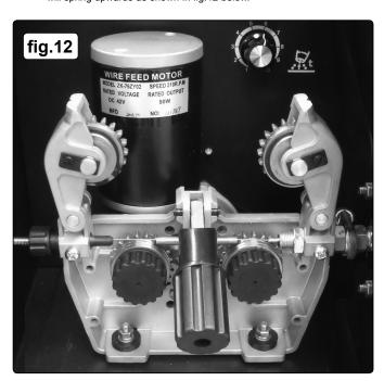
6.2 The wire drive unit is supplied with two pairs of rollers. One pair has drive grooves for Ø0.8mm and Ø1.0mm wire. The second pair has drive grooves for Ø1.0mm and Ø1.2mm.
