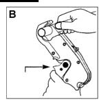
SQUEEZE TRIGGER HANDLE REPEATEDLY TO PIERCE AND CUT THROUGH THE PIPE
