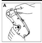
PLACE PLASTIC PIPE INTO 'U' JAW WITH THE BLADE POINT ALIGNED WITH THE TUBE CENTRE
