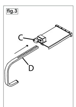
2.3 Turn the key in the lock "C" fully anti-clockwise, to enable the insertion of the locking bar "D" (fig.3).
