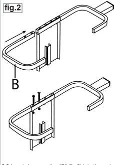
2.2 Insert clamp section "B" (fig.2) into the main plate and secure with supplied nuts and bolts.
