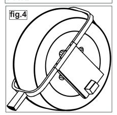
2.4 Take the wheel clamp and place it over the wheel, with the locking plate facing outwards, as in fig.4.
