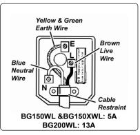
d)After wiring, check that there are no bare wires, that all wires have been correctly connected, that the cable outer insulation extends beyond the cable restraint and that the restraint is tight. Double insulated products, which are always marked with this symbol, are fitted with live (brown) and neutral (blue) wires only. To rewire, connect the wires as indicated above - **DO NOT** connect either wire to the earth terminal.
