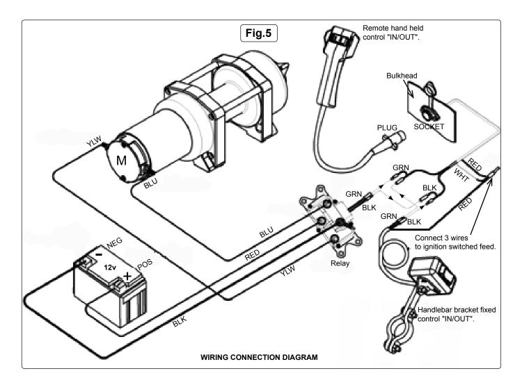
Connect the yellow wire to the positive terminal of the winch, marked as (1) on the rear of the motor case, and to the yellow marked terminal of the relay block. Connect the blue wire to the negative terminal on the winch, marked as (2), to the blue terminal on the relay block. See fig.5.
