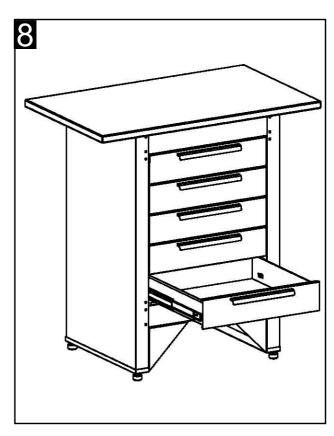
STEP 8. Pull the middle slide and the ball bearings out as far as possible. Hold the drawer and slot the inner slide on the drawer into the middle slide, then push the drawer all the way in.
