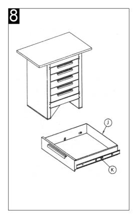
**STEP 8**. Attach a left hand female slide (K) to left hand side of each draw and a right hand female slide (K) to the right hand side of each draw (see diagram 9). Engage each draw onto the protruding male slides and push fully home, then open the draw to check that it is retained.
