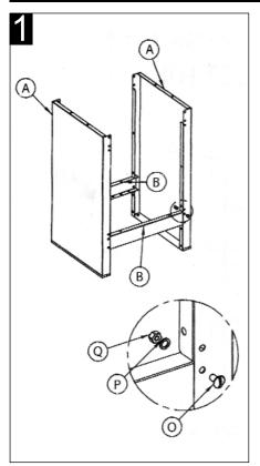
**STEP 1**. Take two crossrails (B) and bolt them to the cabinet sides (A) using 8 bolts (O), 8 lock washers (P), and 8 nuts (Q). Ensure that the pairs of holes that accept the corner braces are facing downwards. (Refer to STEP 5.)
