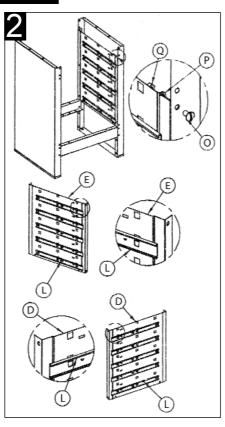
**STEP 2.** Bolt 1 left & 1 right slide panels (D) & (E) into position, only bolt at front of Work Bench using 4 bolts (O), 4 lock washers (P), and 4 nuts (Q). Fix 5 left hand female slide (L), onto each slide panel (D) and 5 right hand female slide (L), onto each slide panel (E) **Refer to Diagram 9 on how to fit slides.**
