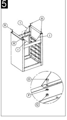
**STEP 4**. Take two crossrails (B) and bolt them to the cabinet sides (A) using 8 bolts (O), 8 lock washers (P), and 8 nuts (Q).
