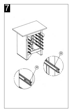
**STEP 7**. Take the 10 male slide components (M) and slide 5 onto the female slides on the left of the draw compartment and 5 onto the female slides on the right hand side of the draw compartment. Push them fully in to engage them, then pull them out to the stop point.
