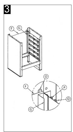
**STEP 3**. Take two draw stops (G) and back panel (F) and bolt them to the back of the cabinet with the draw stops between the panel and the cabinet. Use 4 bolts (O), 4 lock washers (P), and 4 nuts (Q).
