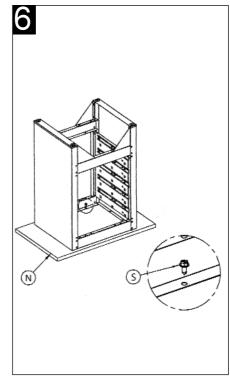
**STEP 6.** Place the wooden top (N) face down on a flat, clean, smooth surface. Position the cabinet upside down on the wooden top and mark the hole locations on the top. Move the cabinet to one side and drill  $5/32^{\circ}$  diameter x  $1/2^{\circ}$  deep holes in the top. DO NOT DRILL DEEPER THAN  $1/2^{\circ}$ . Attach frame to top with the 4 hex head screws (S).
