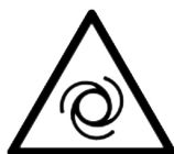
Unexpected Start Up
